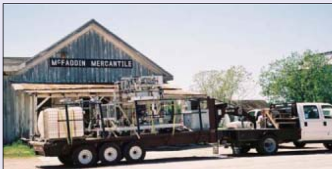
Researchers at the Global Petroleum Research Institute at Texas A&M University built a mobile pretreatment and desalination unit to extract fresh water in the treatment and recycling of water used in hydraulic fracturing. Photo from David Burnett of Texas A&M.
