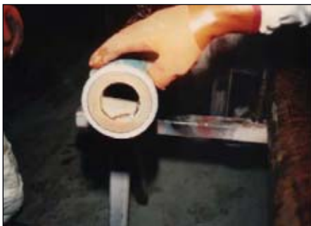
This scale contains a buildup of NORM (Fig. 3; photo from Normcan).
