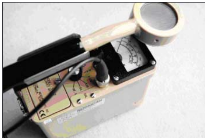
The project employed this Ludlum 3097 Scintillator and an external 44-9 Geiger-Mueller pancake probe (Fig. 4; photo from Normcan).
